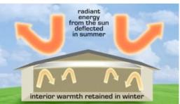
system R-Value of 11.6. The Green Zone works by deflecting heat away in the summer and reflecting heat back into the house during the winter. Traditional mass insulation only slows down heat transfer but the Green Zone combines an R-Value with a dualreflective shield that redirects 97% of the heat that it comes into contact with.
